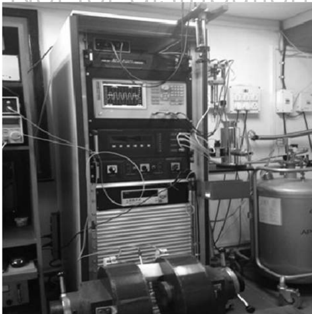
FIGURES 15.4 Measurement of fabric properties on dielectric broadband spectrometer.
