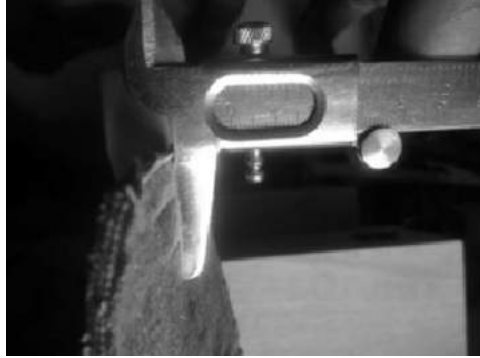
FIGURE 15.6 Thickness measurement on Vernier caliper.
